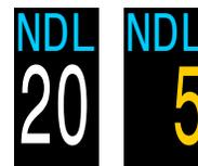
The time remaining, in minutes, at the current depth until decompression stops will be necessary. Displays in **Yellow** when the NDL is less than the low NDL limit (Default 5 minutes).
