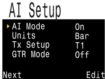
When **AI Mode** is set to **Off**, the AI sub-system is completely powered down and does not consume any power. When on, the AI system increases power consumption by approximately 10%.
